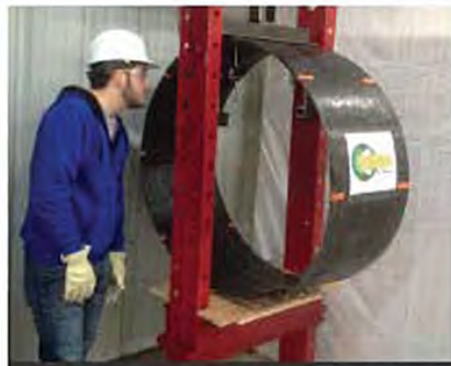
StifPipe® being tested under parallel plate loading (ASTM D2412)
